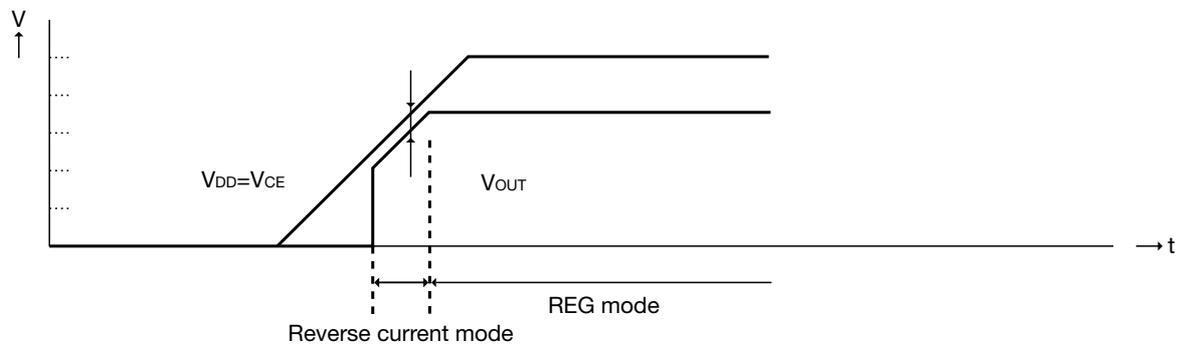
While voltage is building up in the input side, this IC operates in the reverse current mode when  $\Delta V$  (Difference between input and output voltages) is 30mV (Reverse current mode threshold voltage) or less.
