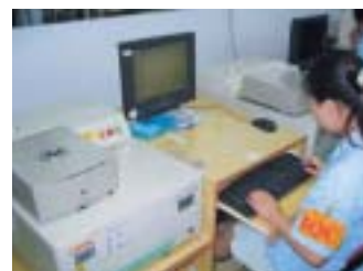
EDXRFによる化学物質含有調査 Inspection of use/nonuse of chemical substances with the EDXRF
