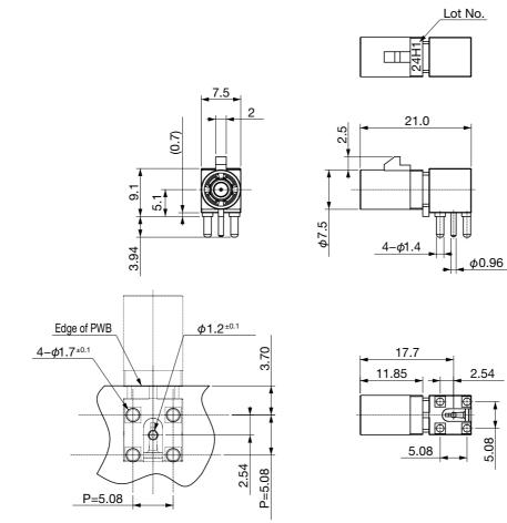
The reference PWB size. (TOLERANCE:±0.05)
