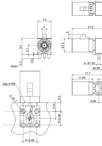
The reference PWB size. (TOLERANCE:±0.05)
